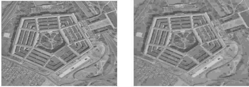
Figure.1. Left: Original image size 512x512; Right: Reconstructed image using 10000 largest magnitude coefficients
